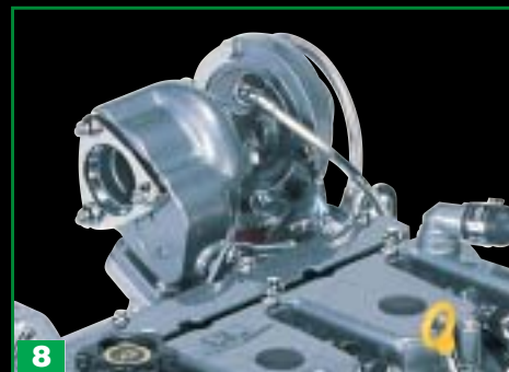
8 Turbocompressore in alto. High Mounted Turbocharger.
